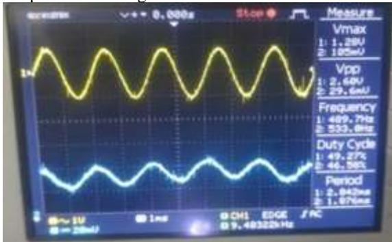
Figure 6. Measurement results on the oscilloscope on the Receiver circuit
